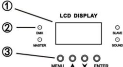
Press the **MENU** button to return, or wait for one minute and then exit the menu mode automatically. When there is no power connection, press the **UP** button for 1 minute to enter the menu mode. After setting, press **MENU** button or wait for 1 minute to exit the power-off setting function automatically.
