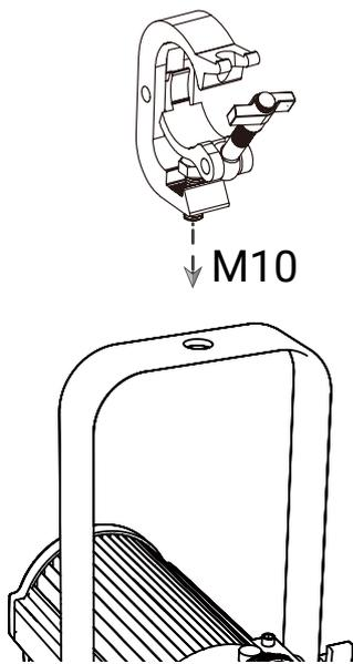
To clamp the fixture to a truss:
