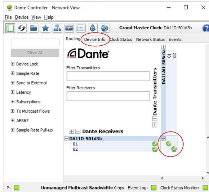
By default the DA11AEN is shipped with its network settings set to obtain an IP Address automatically. This means that if a DHCP server is present on your network, it will provide the DA11AEN with an IP Address. If no DHCP server is present then the DA11AEN will receive a default IP Address in the 169.254.xxx.xxx range. To change the IP Address of the DA11AEN, you must enter the “Network Config” menu in the “Device Info” screen of the Dante Controller software.
